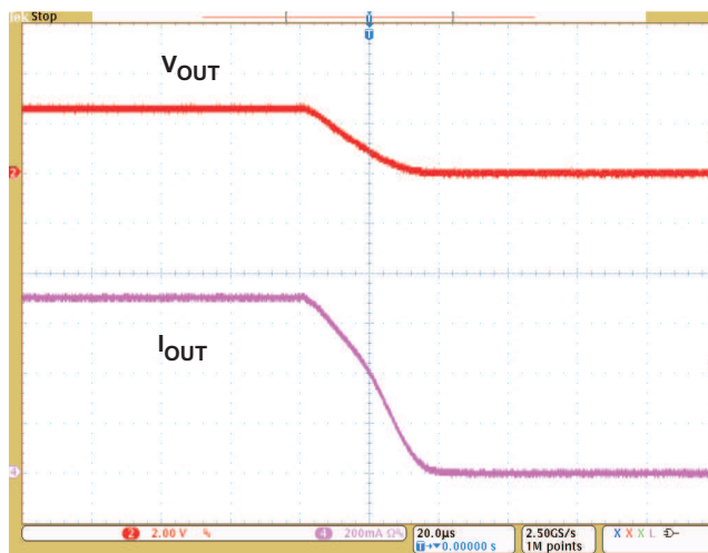
Figure 12. Zoom-in on Turn-off Region of Figure 11, Showing Soft-Stop
