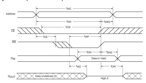
Write Cycle No. 1 ( $\overline{\text{WE}}$ -Controlled) <sup>1,2,3</sup>
