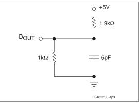
Figure 5. Output Load B
