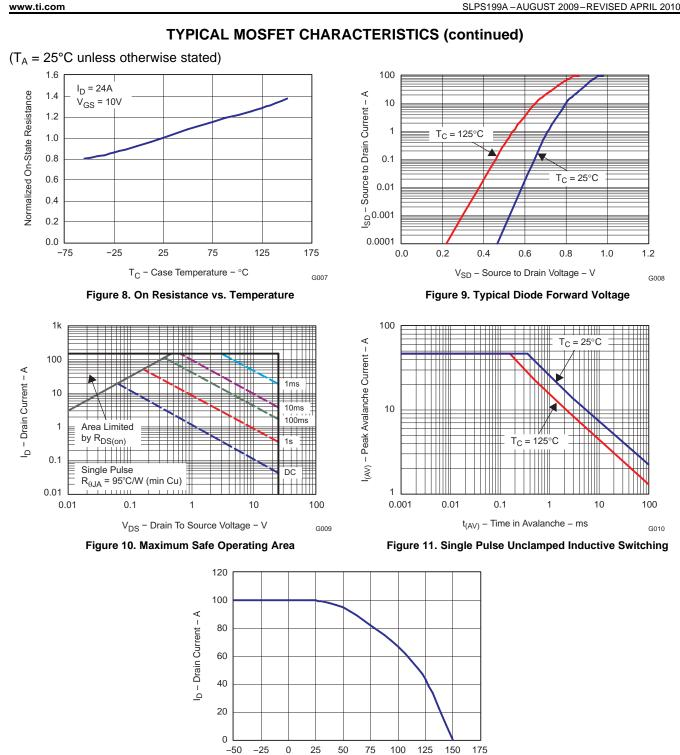
T<sub>C</sub> – Case Temperature – °C G011 Figure 12. Maximum Drain Current vs. Temperature
