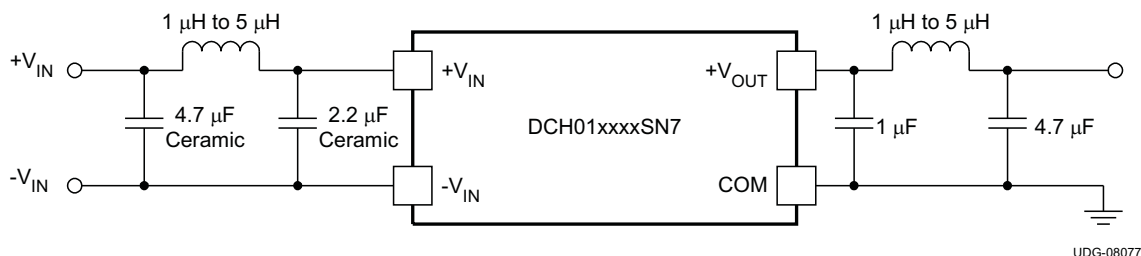
Figure 20. DCH01 Series \pi Filter
