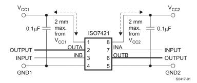
Figure 6. Typical ISO7421x Application Circuit
