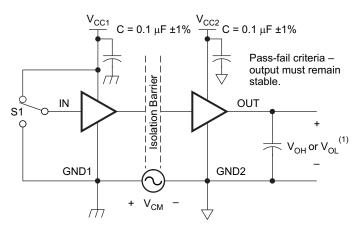
(1)  $C_L = 15 \text{ pF}$  and includes instrumentation and fixture capacitance within  $\pm 20\%$ .
