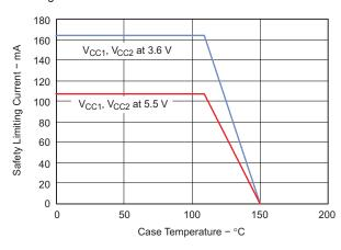
Figure 5.  $\theta_{JC}$  Thermal Derating Curve per IEC 60747-5-2
