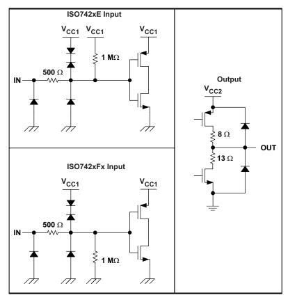
Figure 7. Device I/O Schematics
