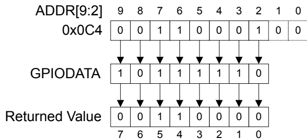
Figure 9-4. GPIODATA Read Example
