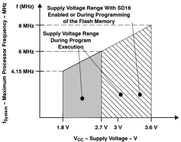
Figure 1. Frequency vs Supply Voltage
