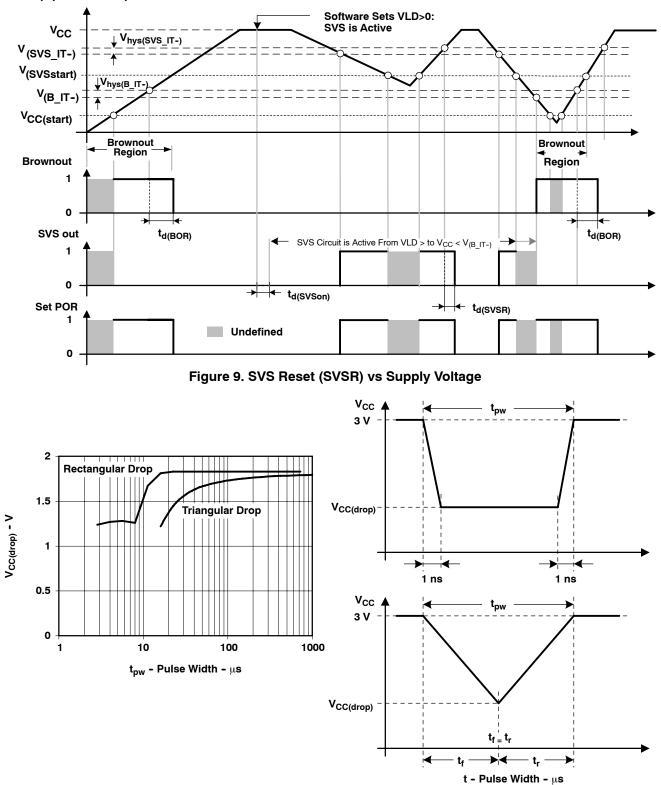
Figure 10. V<sub>CC(drop)</sub> With a Square Voltage Drop and a Triangle Voltage Drop to Generate an SVS Signal
