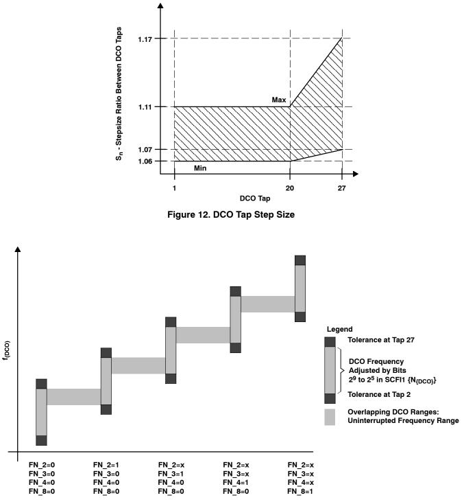
Figure 13. Five Overlapping DCO Ranges Controlled by FN\_x Bits
