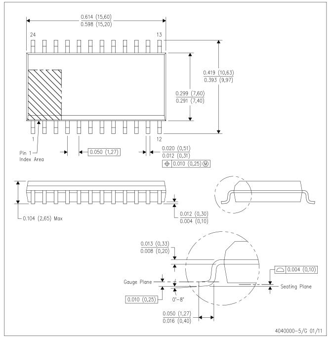
NOTES: A. All linear dimensions are in inches (millimeters). Dimensioning and tolerancing per ASME Y14.5M-1994.
