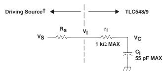
V<sub>I</sub> = Input Voltage at ANALOG IN
