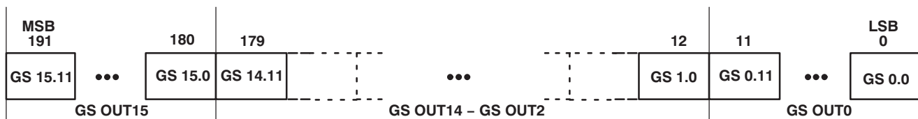
Figure 18. Grayscale Data Packet Format
