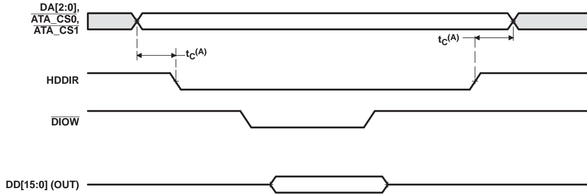
Figure 6-38. ATA/CF HDDIR Taskfile Write/Single PIO Write Timing
