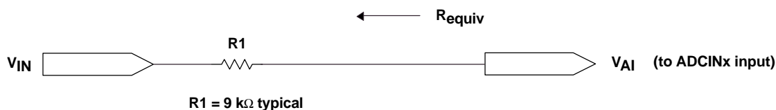
Figure 48. Typical ADC Input Pin Circuit
