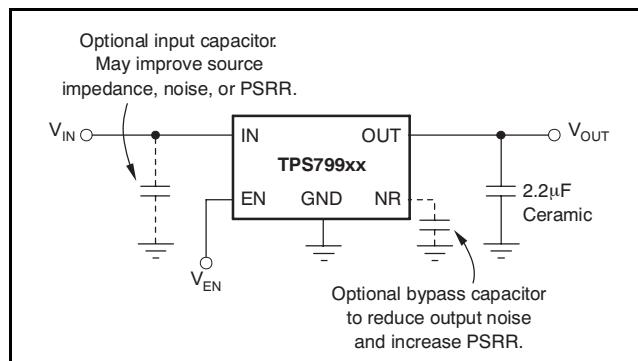
**Figure 28. Typical Application Circuit for Fixed Voltage Versions**
