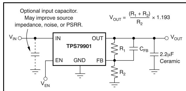
**Figure 29. Typical Application Circuit for Adjustable Voltage Version**
