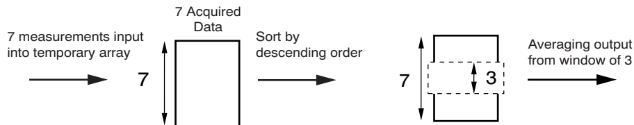
Figure 28. MAV Filter Operation (Patent Pending)
