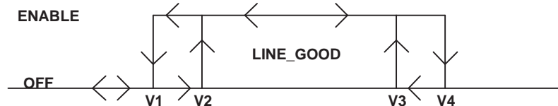
Figure 2. Line UVLO and OVLO Operation
