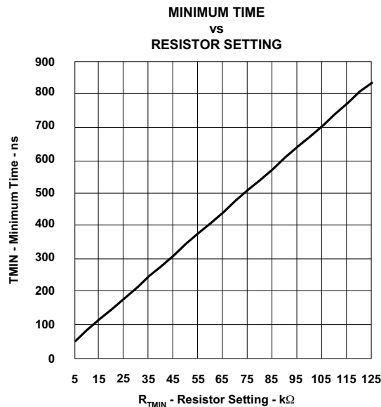
Figure 9. Minimum Time TMIN Over Setting Resistor R_{TMIN}
