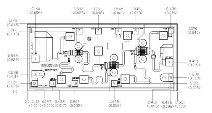
Units: millimeters (inches) Thickness: 0.1016 (0.004)
