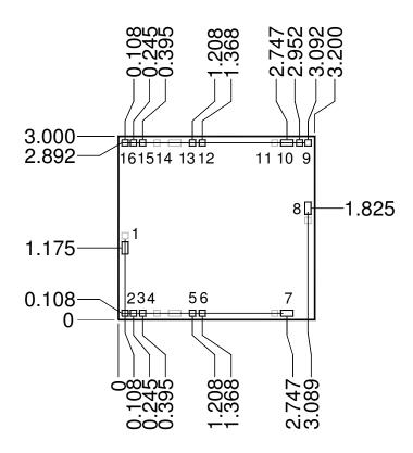
Unit: millimeters Thickness: 0.10
