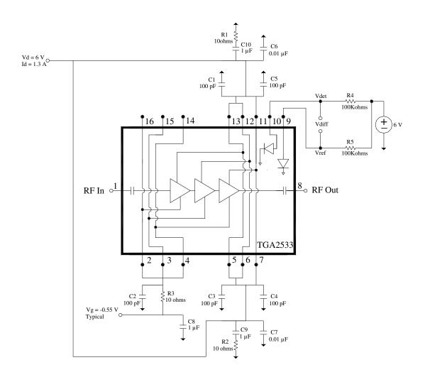
Vg can be biased from either side (pins 2,3,4 or pins 14,15,16), and the non-biased side can be left open. Vd must be biased from both sides (pins 5, 6, 7 and pins 11,12,13).
