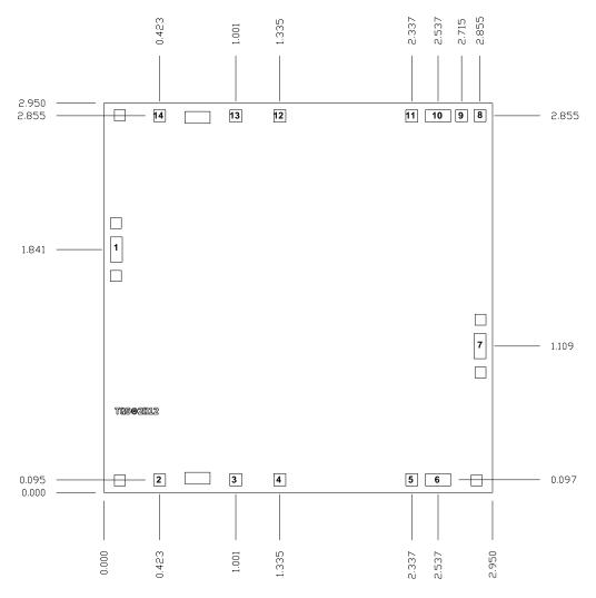
Unit: millimeters Thickness: 0.10
