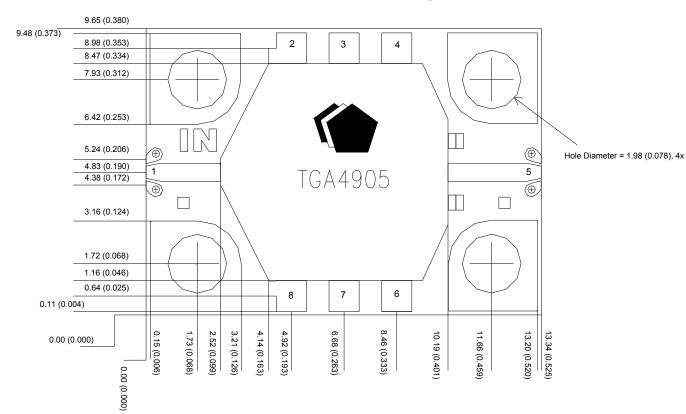
Units: millimeters (inches) Tolerance: +/-0.08 (0.003) RF Ground through Backside
