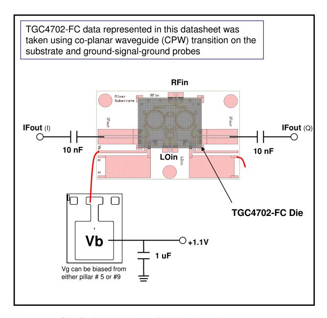
Die is flip-chip soldered to a 15 mil thick alumina test substrate
