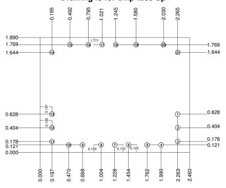
Units: millimeters Thickness: 0.380
