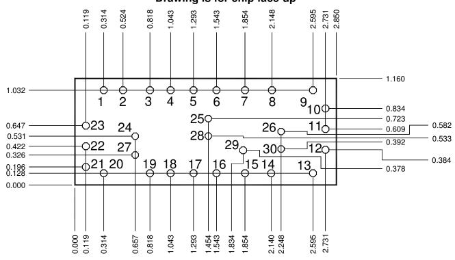
Units: millimeters Thickness: 0.380
