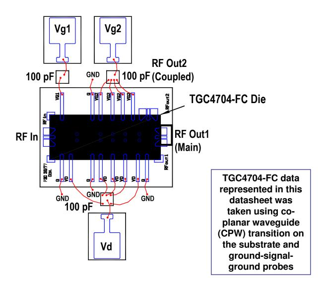
Die is flip-chip soldered to a 15 mil thick alumina test substrate
