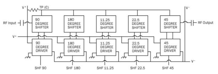
Control voltage inputs should be 0.0 to 0.3 V for logic "0" and 4.5 to 5.3 V for logic "1"
