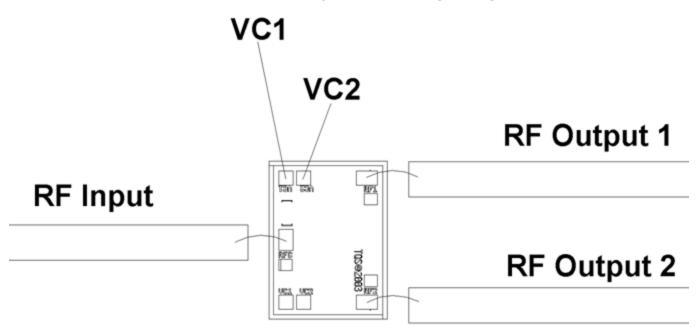
For optimum insertion loss and return loss, a single 0.001" bondwire of length 35 mils should be used. This will be approximately 0.42nH. Differences in bondwire length will have an impact on switch performance.
