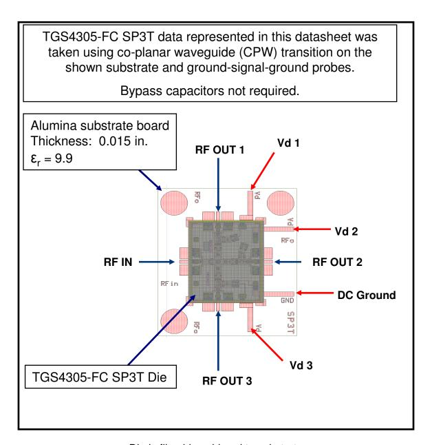
Die is flip-chip soldered to substrate
