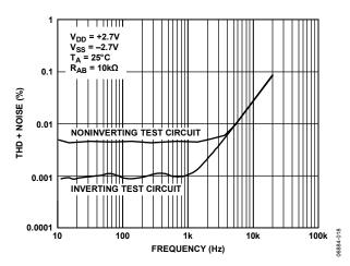
Figure 20. Total Harmonic Distortion Plus Noise vs. Frequency
