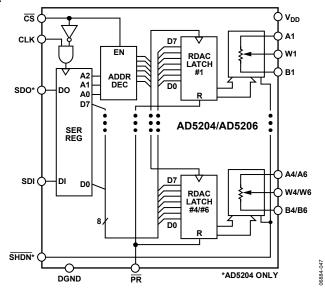
Figure 22. Block Diagram
