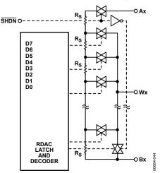
Figure 21. AD5204/AD5206 Equivalent RDAC Circuit
