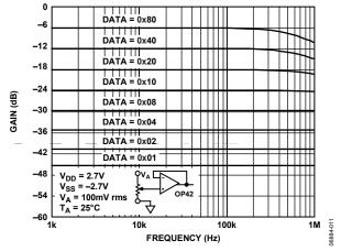
Figure 13. Bandwidth vs. Code,  $10 \, k\Omega$  Version
