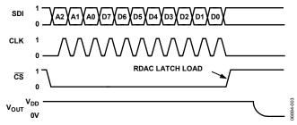
Figure 3. Timing Diagram
