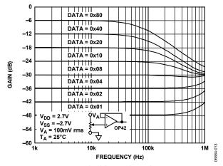
Figure 15. Bandwidth vs. Code, 100  $k\Omega$  Version
