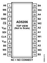
Figure 8. AD5206 SOIC/TSSOP/PDIP Pin Configuration
