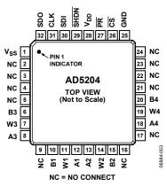
Figure 7. AD5204 LFCSP Pin Configuration
