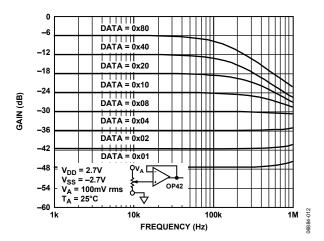
Figure 14. Bandwidth vs. Code,  $50 \, k\Omega$  Version
