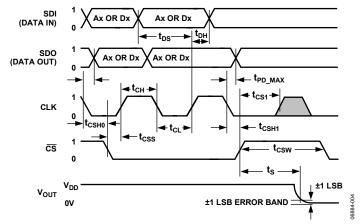
Figure 4. Detailed Timing Diagram
