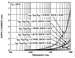
Figure 18. Supply Current vs. Clock Frequency
