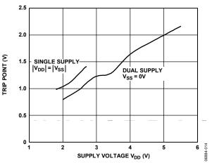
Figure 16. Digital Input Trip Point vs. Supply Voltage
