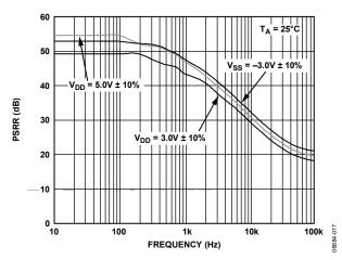
Figure 19. Power Supply Rejection vs. Frequency
