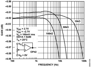
Figure 10. Gain Flatness vs. Frequency
