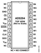
Figure 6. AD5204 SOIC/TSSOP/PDIP Pin Configuration
