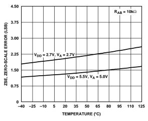
Figure 14. Zero-Scale Error vs. Temperature
