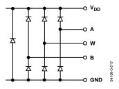
Figure 41. Maximum Terminal Voltages Set by V<sub>DD</sub> and GND
