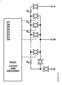
Figure 37. AD5243 Equivalent RDAC Circuit
