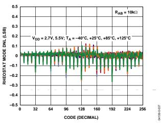
Figure 12. R-DNL vs. Code vs. Temperature
