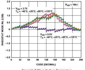
Figure 11. R-INL vs. Code vs. Temperature
