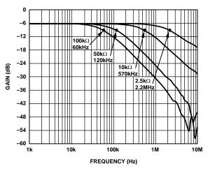
Figure 22. -3 dB Bandwidth @ Code = 0x80
