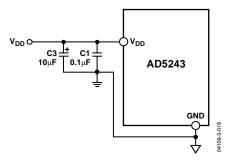
Figure 42. Power Supply Bypassing
