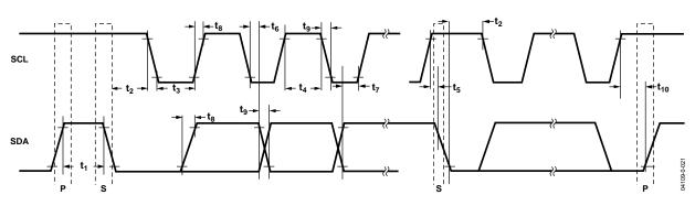
Figure 45. I<sup>2</sup>C Interface Detailed Timing Diagram
