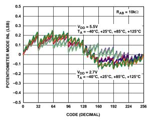
Figure 7. INL vs. Code vs. Temperature
