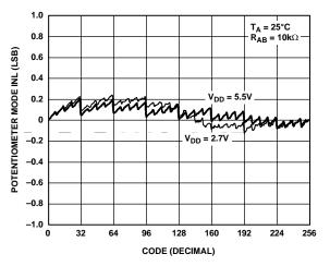
Figure 9. INL vs. Code vs. Supply Voltages
