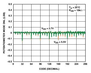
Figure 10. DNL vs. Code vs. Supply Voltages
