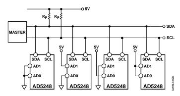
Figure 50. Multiple AD5248 Devices on One I<sup>2</sup>C Bus
