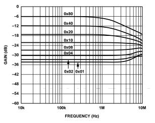
Figure 18. Gain vs. Frequency vs. Code,  $R_{AB} = 2.5 \text{ k}\Omega$
