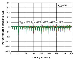
Figure 8. DNL vs. Code vs. Temperature
