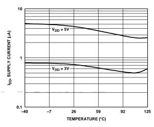
Figure 15. Supply Current vs. Temperature
