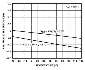
Figure 13. Full-Scale Error vs. Temperature
