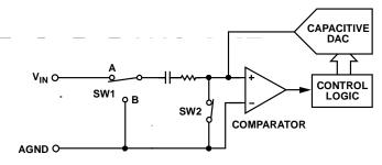
Figure 3 ADC Acquisition Phase
