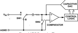
Figure 4 ADC Conversion Phase
