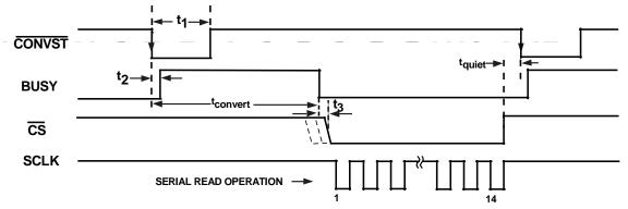
Figure 7. Normal Mode Operation
