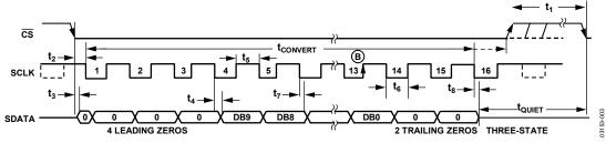
Figure 3. AD7441 Serial Interface Timing Diagram
