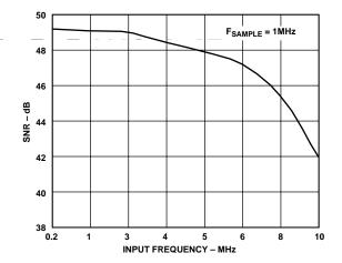
Figure 8. SNR vs. Input Frequency On the AD7827
