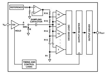
Figure 3. ADC Conversion Phase
