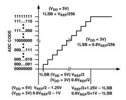
Figure 6. Transfer Characteristic
