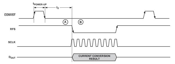
Figure 14. Mode 2 Operation Timing Diagram
