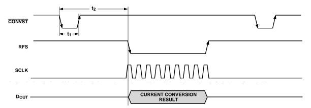
Figure 13. Mode 1 Operation Timing Diagram
