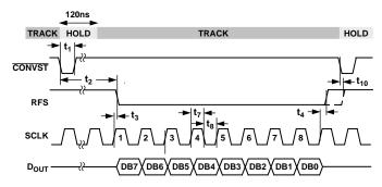
Figure 4. Track-and-Hold Timing
