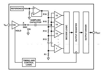
Figure 2. ADC Acquisition Phase
