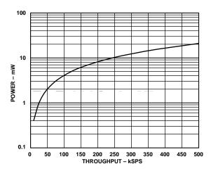
Figure 11. Power vs. Throughput
