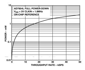
Figure 27. Power vs. Throughput AD7854L
