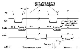
Figure 33. Timing Diagram for Full System Calibration
