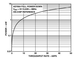
Figure 26. Power vs. Throughput AD7854
