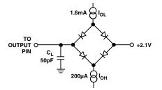
Figure 1. Load Circuit for Digital Output Timing **Specifications**
