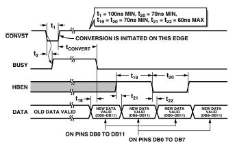
Figure 36. Read Cycle Timing Diagram with  $\overline{CS}$  and  $\overline{RD}$  Tied Low
