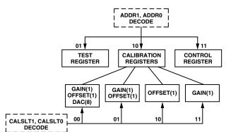
Figure 2. Write Register Hierarchy/Address Decoding
