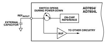
Figure 22. On-Chip Reference During Power-Down
