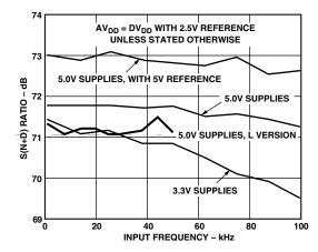
Figure 19. SNR vs. Frequency
