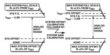
Figure 32. System (Gain + Offset) Calibration
