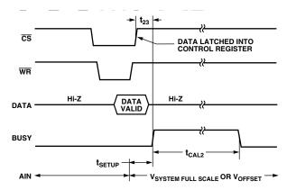
Figure 34. Timing Diagram for System Gain or System Offset Calibration
