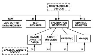
Figure 3. Read Register Hierarchy/Address Decoding
