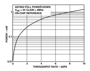
Figure 24. Power vs. Throughput AD7854
