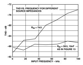
Figure 10. THD vs. Analog Input Frequency
