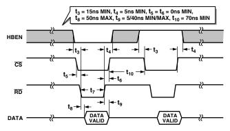
Figure 35. Read Cycle Timing Diagram Using CS and RD
