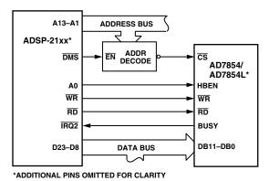
Figure 38. AD7854/AD7854L to ADSP-21xx Parallel Interface
