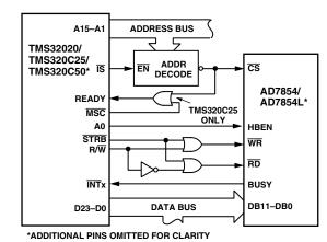
Figure 39. AD7854/AD7854L to TMS32020/C25/C5x
