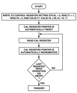
Figure 7. Flowchart for Reading from the Calibration Registers
