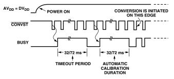
*Figure 28. Timing Arrangement for Autocalibration on Power-On*
