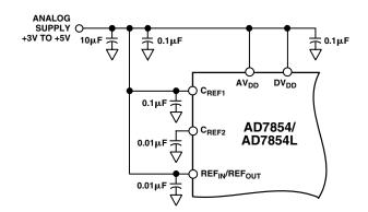
Figure 17. Relevant Connections, AV<sub>DD</sub> as the Reference
