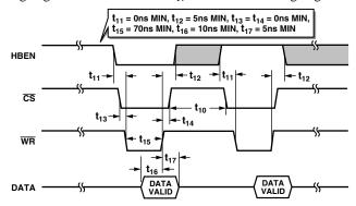
Figure 37. Write Cycle Timing Diagram
