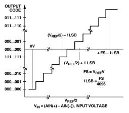
Figure 15. AD7854/AD7854L Bipolar Transfer Characteristic
