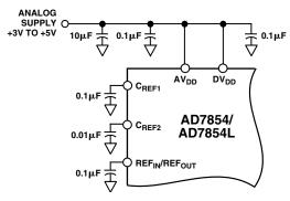
Figure 16. Relevant Connections Using Internal Reference
