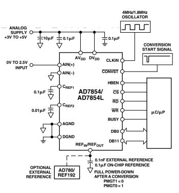
Figure 23. Typical Low Power Circuit
