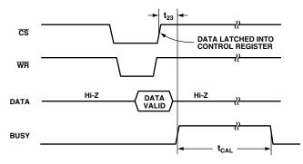
Figure 29. Timing Diagram for Full Self-Calibration
