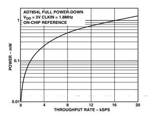
Figure 25. Power vs. Throughput AD7854L
