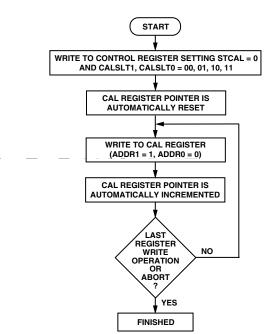
Figure 6. Flowchart for Writing to the Calibration Registers
