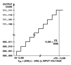
Figure 14. AD7854/AD7854L Unipolar Transfer Characteristic
