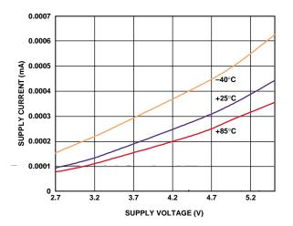
Figure 14. AD7998 Shutdown Current vs. Supply Voltage, -40°C, +25°C, and +85°C
