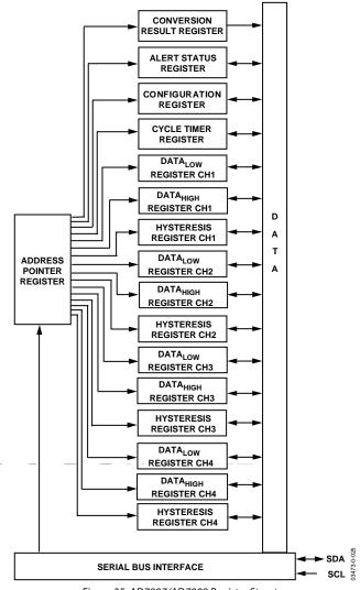
Figure 25. AD7997/AD7998 Register Structure
