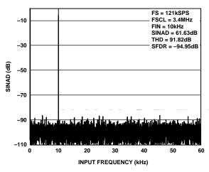
Figure 5. AD7997 Dynamic Performance with 5 V Supply and 2.5 V Reference, 121 kSPS, Mode 1
