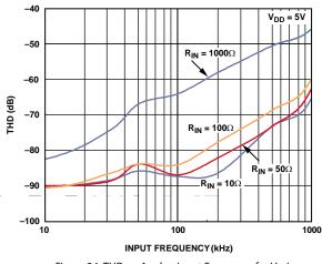
Figure 24. THD vs. Analog Input Frequency for Various Source Impedances for V<sub>DD</sub> = 5 V, 136 kSPS, Mode 1
