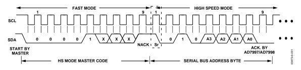
Figure 31. Placing the Part into High Speed Mode
