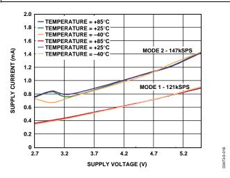
Figure 16. AD7998 Average Supply Current vs. Supply Voltage for Various Temperatures
