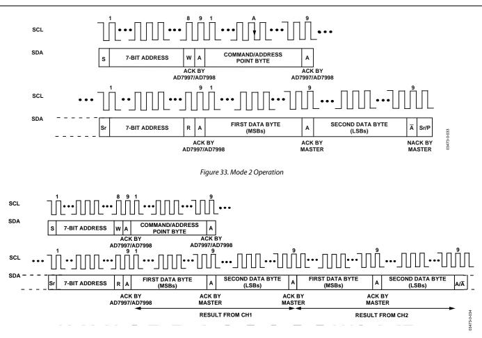
Figure 34. Mode 2 Sequence Operation
