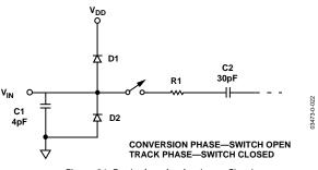
Figure 21. Equivalent Analog Input Circuit
