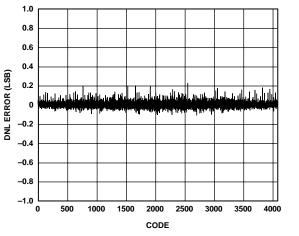
Figure 9. Typical DNL, V<sub>DD</sub> = 5.5 V, Mode 1, 3.4 MHz f<sub>SCL</sub>, 121 kSPS
