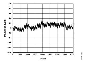
Figure 10. Typical INL,  $V_{DD} = 2.7 V$ , Mode 1, 3.4 MHz f<sub>SCL</sub>, 121 kSPS
