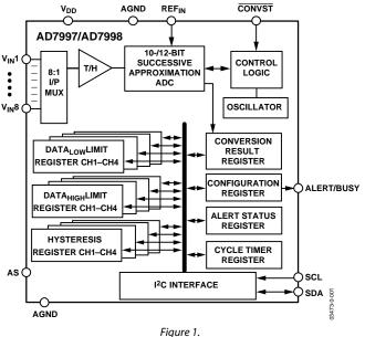
On-chip limit registers can be programmed with high and low limits for the conversion result, and an open-drain, out-ofrange indicator output (ALERT) becomes active when the programmed high or low limits are violated by the conversion result. This output can be used as an interrupt.
