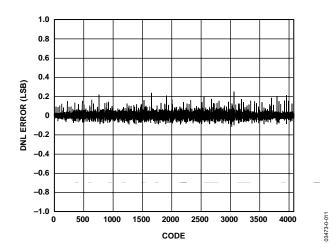
Figure 11. Typical DNL,  $V_{DD} = 2.7 V$ , Mode 1, 3.4 MHz f<sub>SCL</sub>, 121 kSPS
