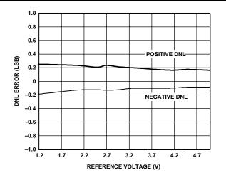
Figure 13. AD7998 Change in DNL vs. Reference Voltage  $V_{DD} = 5 V$ , Mode 1, 121 kSPS
