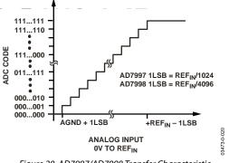
Figure 20. AD7997/AD7998 Transfer Characteristic
