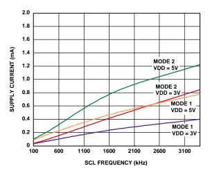
Figure 15. AD7998 Average Supply Current vs. I<sup>2</sup>C Bus Rate for  $V_{DD}$  = 3 V and 5 V
