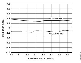
Figure 12. AD7998 Change in INL vs. Reference Voltage  $V_{DD} = 5 V$ , Mode 1, 121 kSPS
