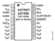
Figure 3. AD7998/AD7997 Pin Configuration
