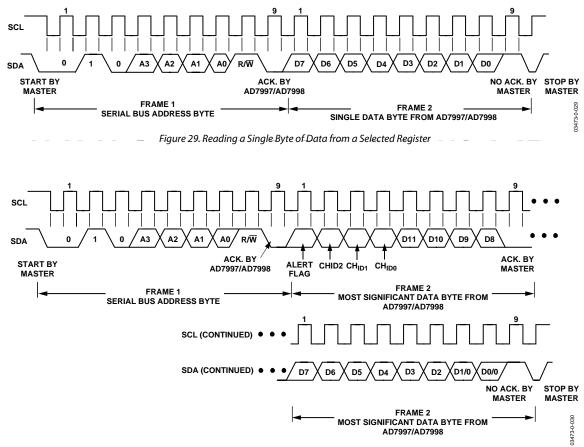
Figure 30. Reading Two Bytes of Data from the Conversion Result Register
