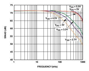
Figure 7. AD7998 SINAD vs. Analog Input Frequency for Various Supply Voltages, 3.4 MHz fsci, 136 kSPS
