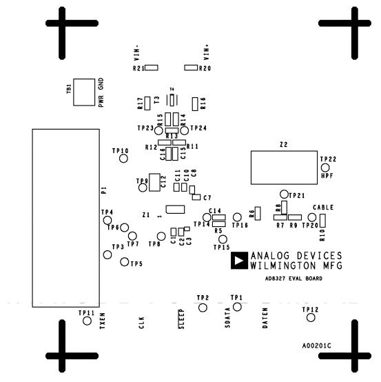
Figure 11. Evaluation Board Layout—Top Silkscreen
