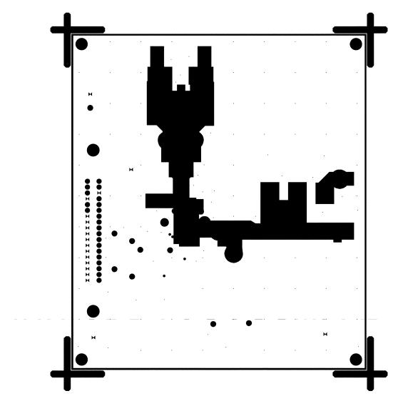
Figure 13. Evaluation Board Layout—Internal Ground Plane
