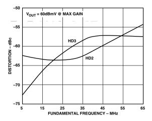
Figure 1. Harmonic Distortion vs. Frequency
