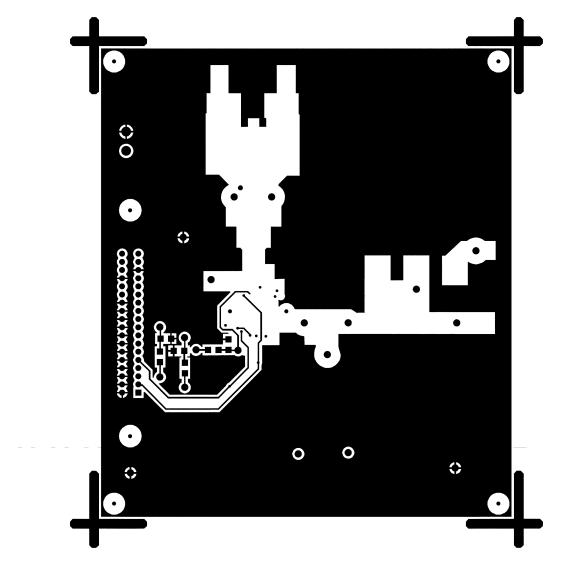
Figure 15. Evaluation Board Layout—Circuit Side
