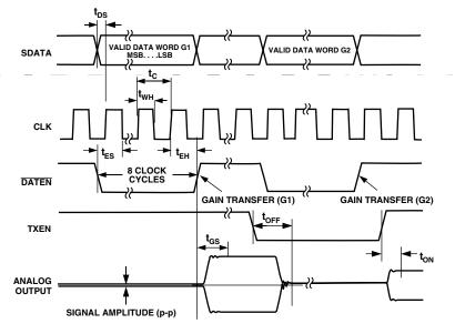
Figure 2. Serial Interface Timing
