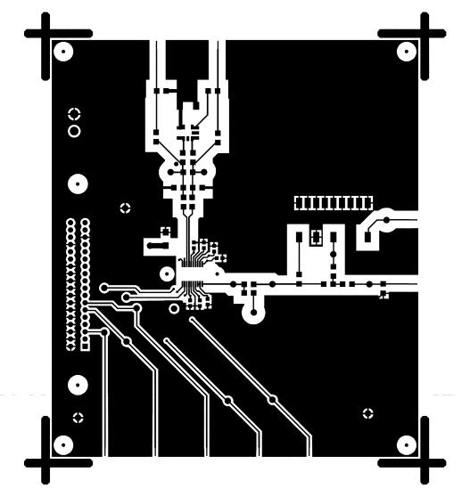
Figure 12. Evaluation Board Layout—Component Side
