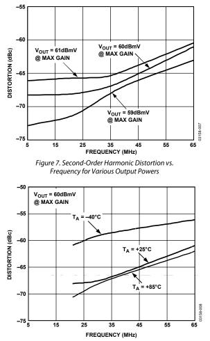
Figure 8. Second-Order Harmonic Distortion vs. Frequency vs. Temperature
