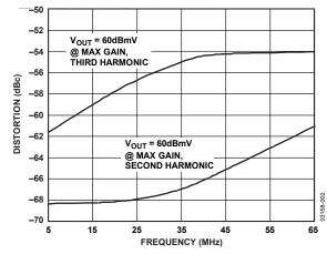
Figure 2. Worst Harmonic Distortion vs. Frequency
