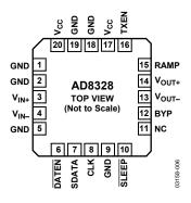
Figure 6. 20-Lead LFCSP Pin Configuration
