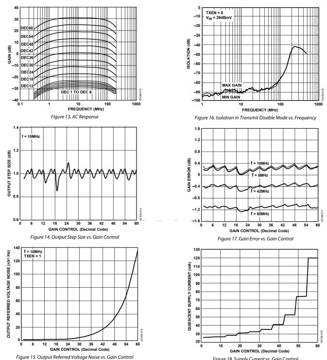
Figure 18. Supply Current vs. Gain Control
