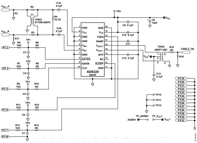
Figure 26. AD8328 Evaluation Board Schematic
