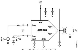
Figure 19. Characterization Circuit
