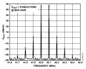
Figure 12. Two-Tone Intermodulation Distortion
