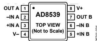
Figure 4. 8-Lead MSOP (RM-8)
