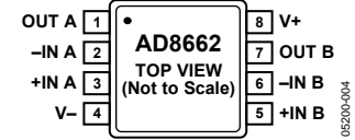
Figure 4. AD8662, 8-Lead MSOP (RM-8)
