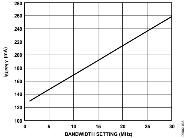
Figure 38. Current Consumption vs. Bandwidth Setting (Gain = 20 dB)
