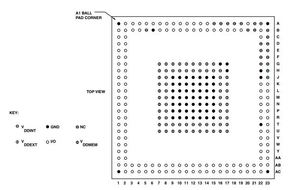
Figure 65. 289-Ball CSP\_BGA Ball Configuration (Top View)
