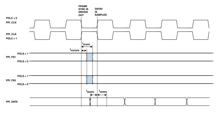
Figure 21. PPI GP Rx Mode with Internal Frame Sync Timing
