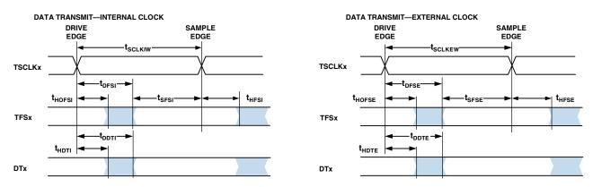
NOTE: EITHER THE RISING EDGE OR FALLING EDGE OF RSCLKX OR TSCLKX CAN BE USED AS THE ACTIVE SAMPLING EDGE.
