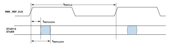
Figure 37. 10/100 Ethernet MAC Controller Timing: RMII Transmit Signal
