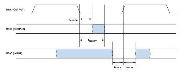
Figure 39. 10/100 Ethernet MAC Controller Timing: MII Station Management
