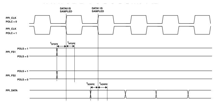
Figure 19. PPI GP Rx Mode with External Frame Sync Timing
