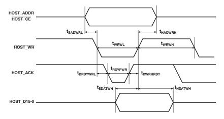
Figure 33. HOSTDP A/C- Host Write Cycle
