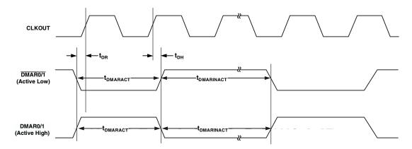
Figure 18. External DMA Request Timing
