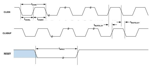
Figure 9. Clock and Reset Timing
