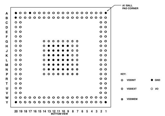
Figure 68. 208-Ball CSP\_BGA Ball Configuration (Bottom View)
