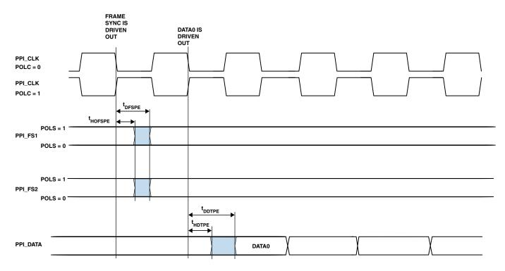
Figure 22. PPI GP Tx Mode with Internal Frame Sync Timing
