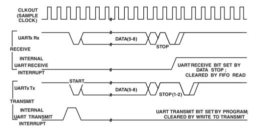
Figure 27. UART Ports—Receive and Transmit Timing
