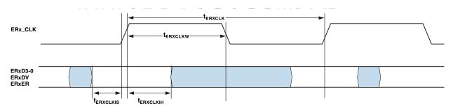
Figure 34. 10/100 Ethernet MAC Controller Timing: MII Receive Signal
