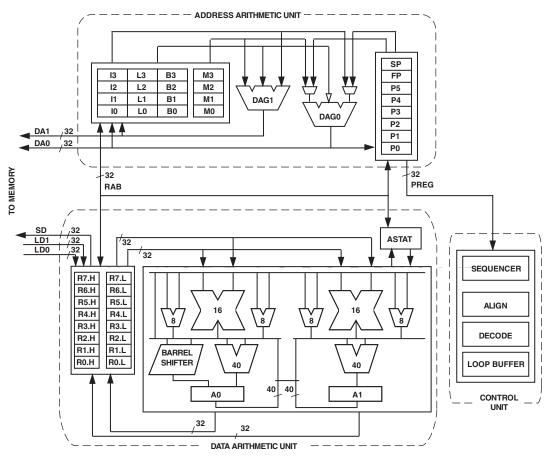
Figure 2. Blackfin Processor Core
