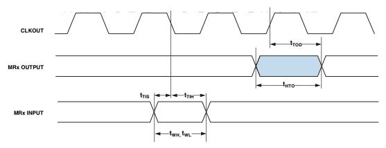
Figure 29. Timer Cycle Timing
