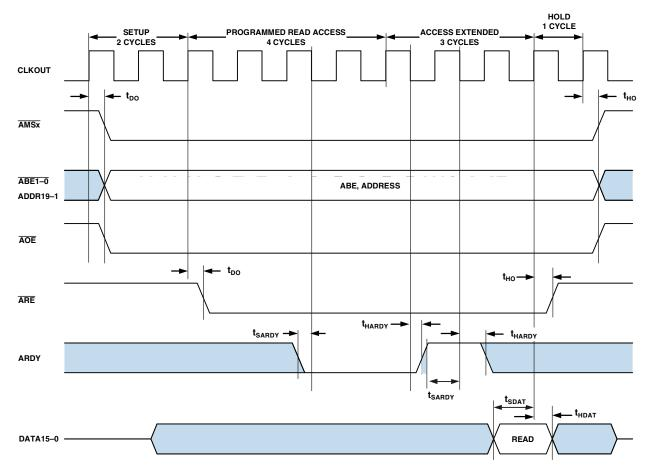
Figure 10. Asynchronous Memory Read Cycle Timing
