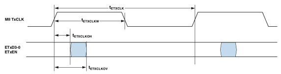
Figure 35. 10/100 Ethernet MAC Controller Timing: MII Transmit Signal
