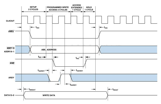
Figure 11. Asynchronous Memory Write Cycle Timing
