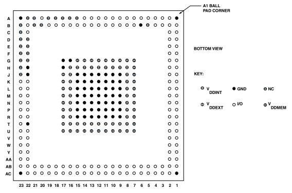
Figure 66. 289-Ball CSP\_BGA Ball Configuration (Bottom View)
