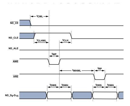
Figure 16. NAND Flash Controller Interface Timing - Write Followed by Read Operation
