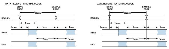
NOTE: EITHER THE RISING EDGE OR FALLING EDGE OF RSCLKX OR TSCLKX CAN BE USED AS THE ACTIVE SAMPLING EDGE.
