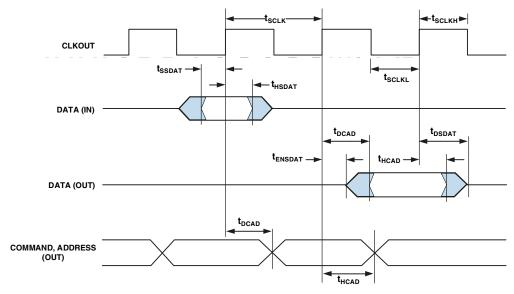
NOTE: COMMAND =  $\overline{SRAS}$ ,  $\overline{SCAS}$ ,  $\overline{SWE}$ , SDQM,  $\overline{SMS}$ , SA10, SCKE.
