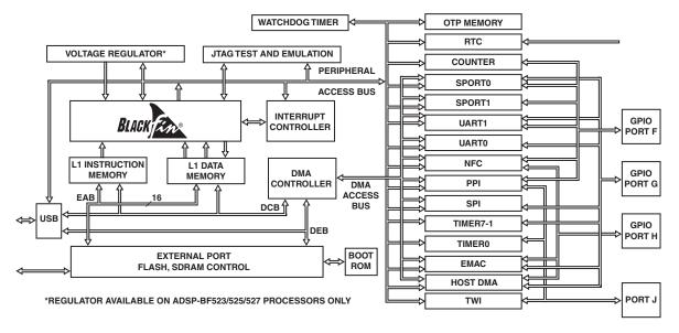
Figure 1. Processor Block Diagram
