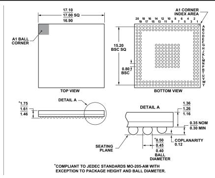
Figure 70. 208-Ball CSP\_BGA (BC-208-2)
