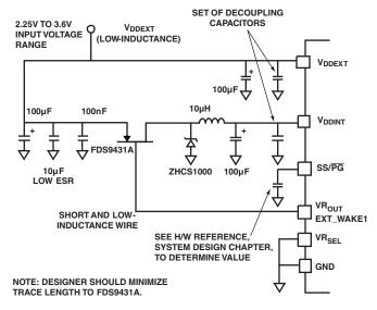
Figure 5. ADSP-BF523/525/527 Voltage Regulator Circuit
