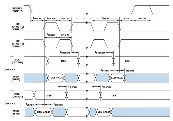
Figure 25. Serial Peripheral Interface (SPI) Port—Master Timing
