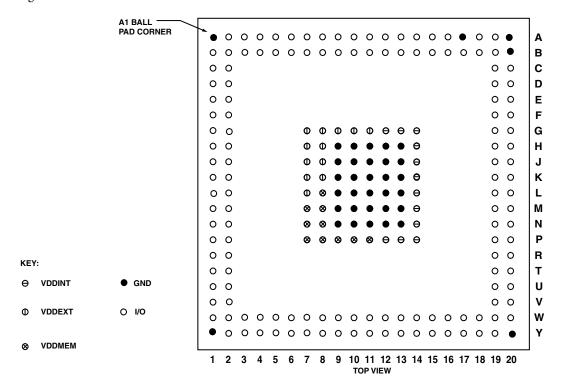
Figure 67. 208-Ball CSP\_BGA Ball Configuration (Top View)
