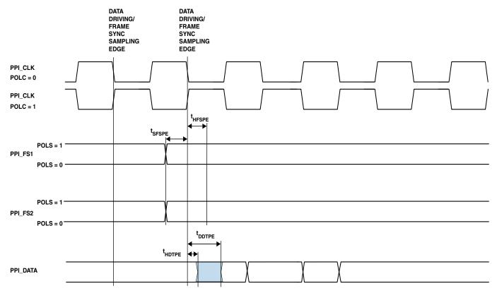
Figure 20. PPI GP Tx Mode with External Frame Sync Timing
