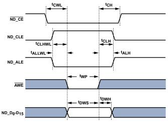
Figure 12. NAND Flash Controller Interface Timing - Command Write Cycle
