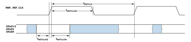
Figure 36. 10/100 Ethernet MAC Controller Timing: RMII Receive Signal
