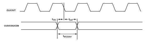
Figure 31. Up/Down Counter/Rotary Encoder Timing
