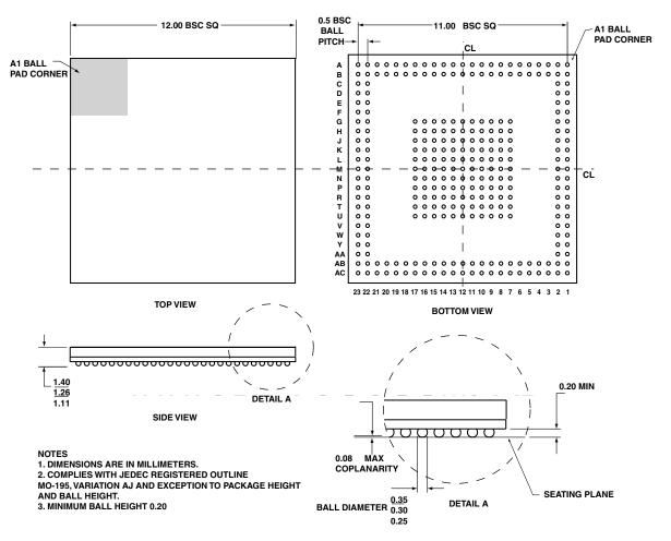
Figure 69. 289-Ball CSP\_BGA (BC-289-2)
