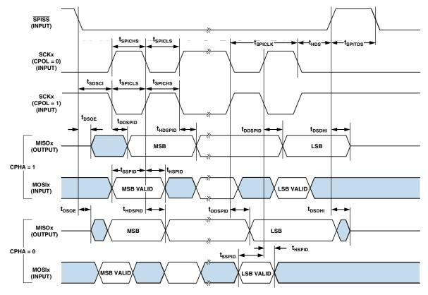
Figure 26. Serial Peripheral Interface (SPI) Port—Slave Timing
