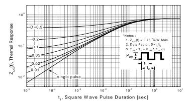
Figure 11-2. Transient Thermal Response Curve (FCPF16N60)
