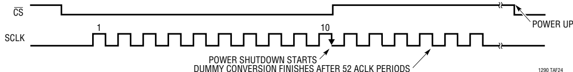
Figure 24. Power Shutdown Timing
