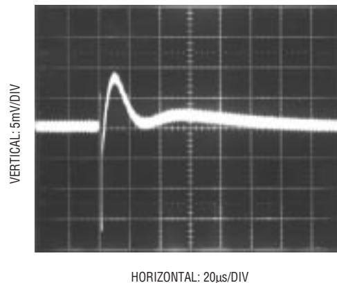
Figure 14. Poor Op Amp Settling Can Cause A/D Errors
