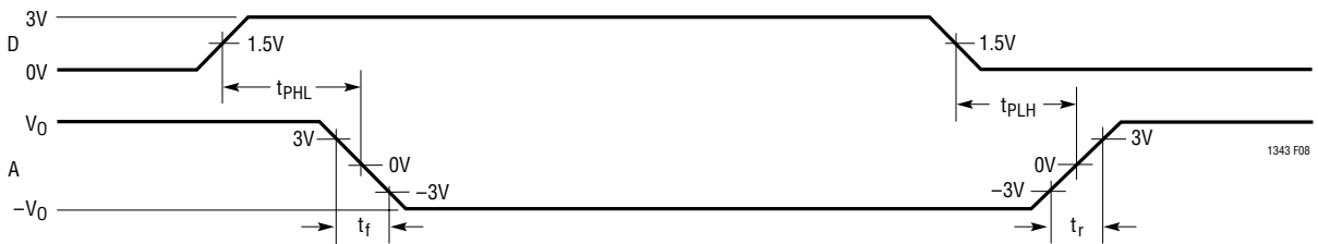
Figure 8. V.10, V.28 Driver Propagation Delays
