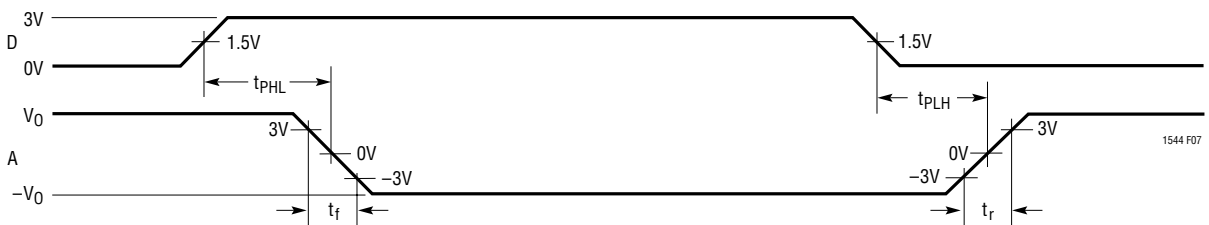
Figure 7. V.10, V.28 Driver Propagation Delays
