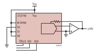
Figure 1. Using M-SPAN to Configure the LTC2756 for Single-Span Operation (±10V Range Shown)
