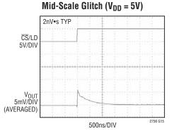
LT1468 AMP;  $C_{FEEDBACK} = 20pF$  OV TO 10V STEP  $V_{REF} = -10V$ ; SPAN CODE = 0000  $t_{SETTLE} = 1.8\mu s$  to 0.0004% (18 BITS)
