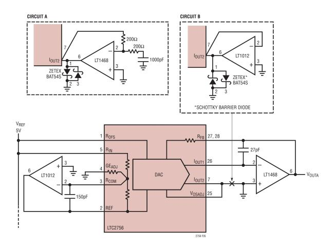
Figure 4. If a Low-Impedance GND Plane Is Unavailable, Drive  $I_{OUT2}$  with a Force/Sense Amplifier As Shown. Use Circuit A to Minimize Impact on Settling Time, or Circuit B for Lower Power Consumption and Better Accuracy
