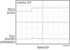
Mid-Scale Glitch  $(V_{DD} = 3V)$
