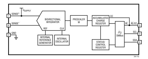
Figure 2. Block Diagram of the LTC2941
