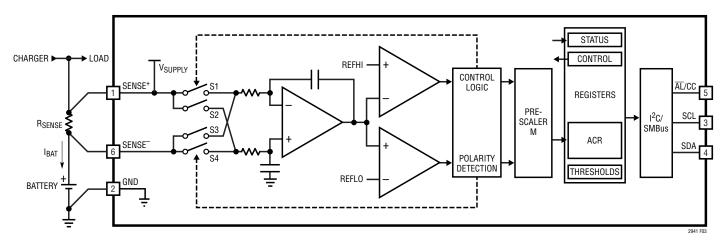
Figure 3. Coulomb Counter Section of the LTC2941
