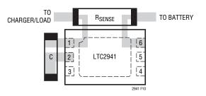
Figure 10. Kelvin Connection on Sense Resistor
