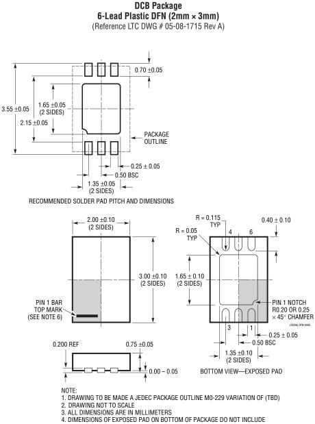
MOLD FLASH. MOLD FLASH, IF PRESENT, SHALL NOT EXCEED 0.15mm ON ANY SIDE 5. EXPOSED PAD SHALL BE SOLDER PLATED
