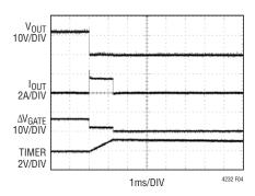
Figure 4. Short-Circuit Waveform
