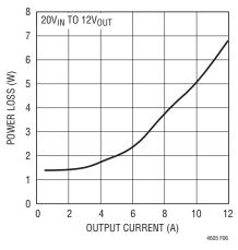
Figure 6.  $20V_{IN}$  Power Loss
