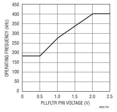
Figure 2. Frequency vs PLLFLTR Pin Voltage
