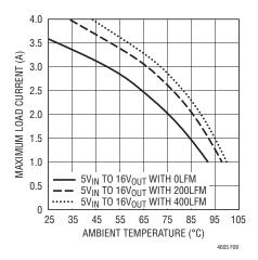
Figure 9.  $5V_{\text{IN}}$  to  $16V_{\text{OUT}}$  without Heat Sink
