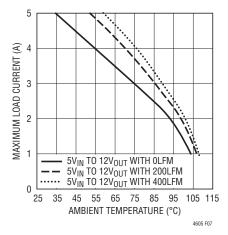
Figure 7.  $5V_{\text{IN}}$  to  $12V_{\text{OUT}}$  without Heat Sink
