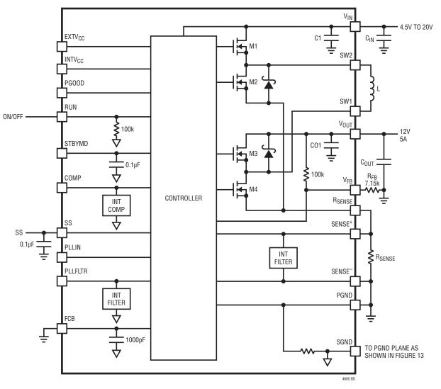
Figure 1. Simplified LTM4605 Block Diagram
