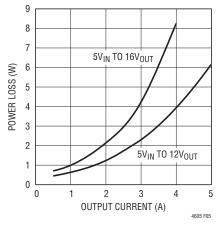
Figure 5.  $5V_{IN}$  Power Loss
