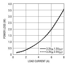
Figure 7. 3.3V  $_{\mbox{IN}}$  , 2.5V and 1.5V  $_{\mbox{OUT}}$  Power Loss
