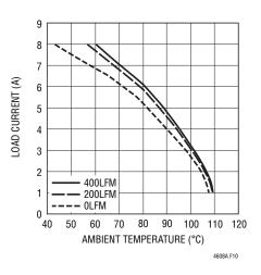
Figure 10. BGA Heat Sink with  $3.3V_{IN}$  to  $1.5V_{OUT}$
