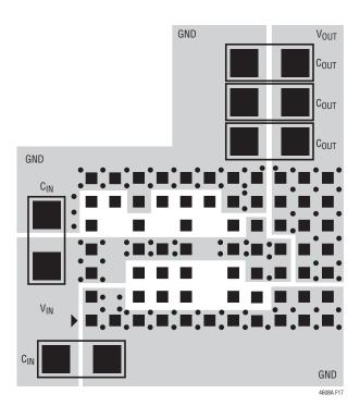
Figure 17. Recommended PCB Layout
