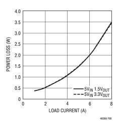
Figure 8.  $5V_{\text{IN}},\,3.3V$  and  $1.5V_{\text{OUT}}$  Power Loss
