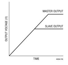
Figure 6. Output Voltage Coincident Tracking
