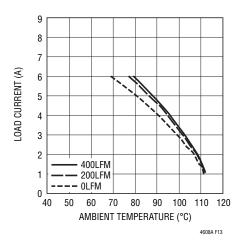
Figure 13. No Heat Sink with  $3.3V_{\text{IN}}$  to  $2.5V_{\text{OUT}}$
