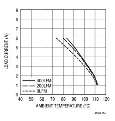
Figure 14. BGA Heat Sink with  $3.3V_{\text{IN}}$  to  $2.5V_{\text{OUT}}$
