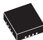
QFN16 (Q) 3 mm x 3 mm
